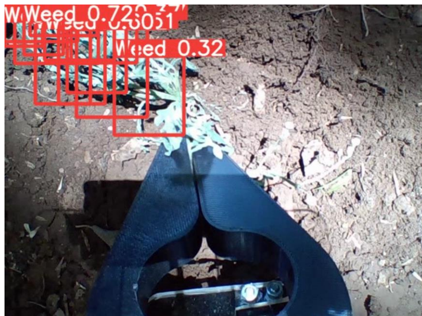
Result obtained from on field testing while integrated with robot. Maximum efficiency 72%.
