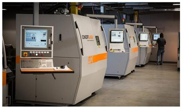
Protolabs uses Concept Laser's Mlab and M2 machines for metal, 3D-printed parts.
