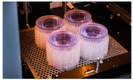
SLA technology forms plastic parts by curing a liquid thermoset resin with a UV laser. As parts are built, they require support structures which are removed once the build completes.
