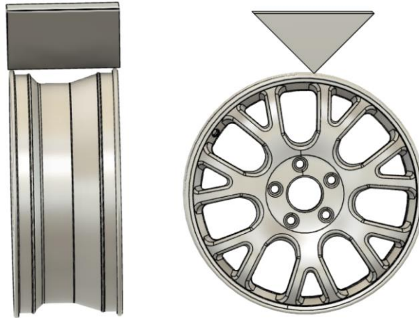
Figure 3. simulation setup of impact load on the wheel rim.
