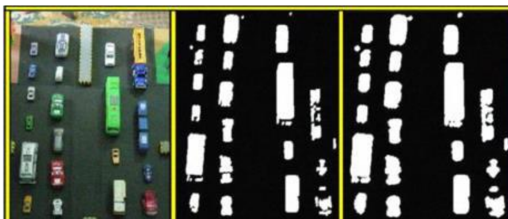
Figure 6 (a) Original image (b) Before applying second level dilation (c) After applying second level dilation.
