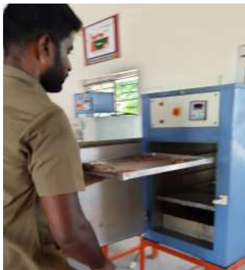
Figure 1 – Measurement of Moisture Content using Hot Air Oven
