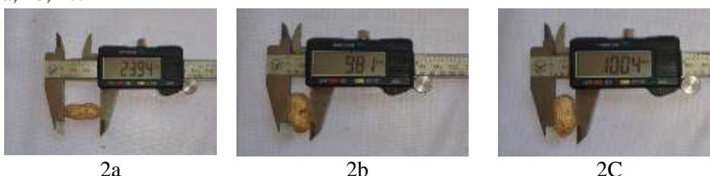
Figure 2a, 2b, 2c – Measurement of Length (L), Width (W) and Thickness (T) using vernier caliper
