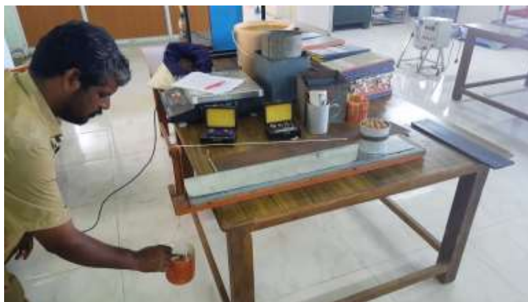
Figure 5 – Measurement of Static Coefficient of Friction using measuring apparatus
