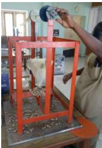
Figure 4 – Measurement of Angle of Repose using measuring apparatus
