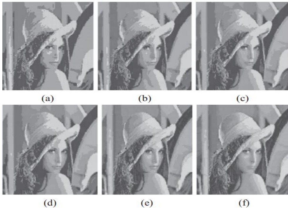
Figure 7. Decompressed Lena image using various algorithms (Codebook size = 256): (a) LBG (b) PSO- LBG, (c) HBMO- LBG (d) FA- LBG (e) BA-LBG (f) Proposed algorithm
