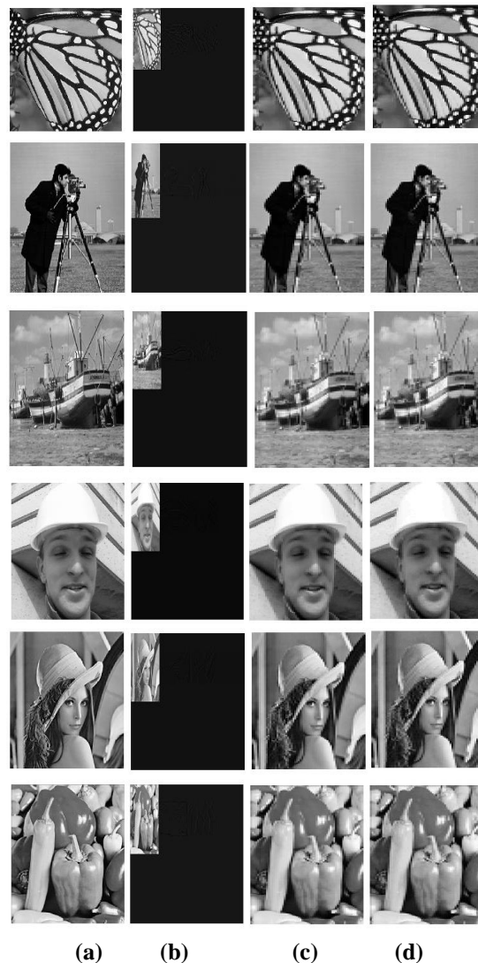
Figure 4 (a) Original Image (tif) 256x256, (b) three level DWT Sub-Image, (c) Image Reconstruction without threshold, (d) Image Reconstruction with threshold
