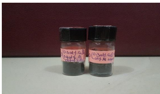
Figure 6. Al and Cu double doped ZnO nanoparticles. First one is 0.3at. % Cu and 0.2at. % Al doped ZnO and other one is 0.5at.% Cu and 0.4.at% Al doped ZnO.
