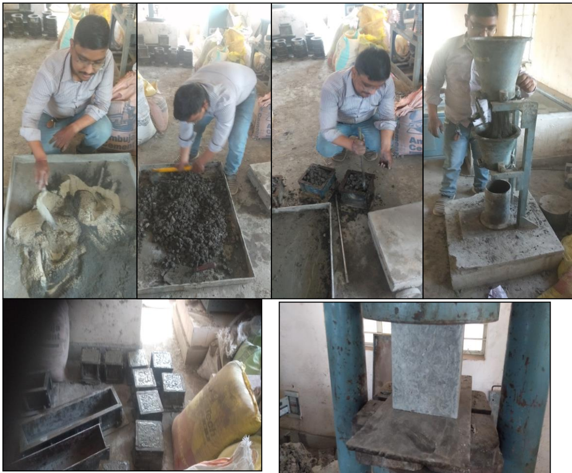
FIGURE 2: Dry Mix, Mixing Of Concrete, Filling In Mould, Compaction Factor, Casted Moulds and Compressive Strength Test
