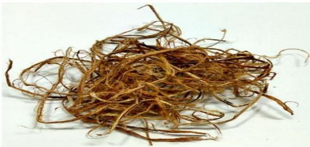
FIGURE 2 Extracted fiber from Bauhinia Vahlia stem [Color figure can be viewed at wileyonlinelibrary.com ]
