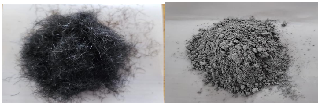
Figure-2:- Chopped Human Beard (Natural fiber) and Ferro chrome slag(Filler Materials)
