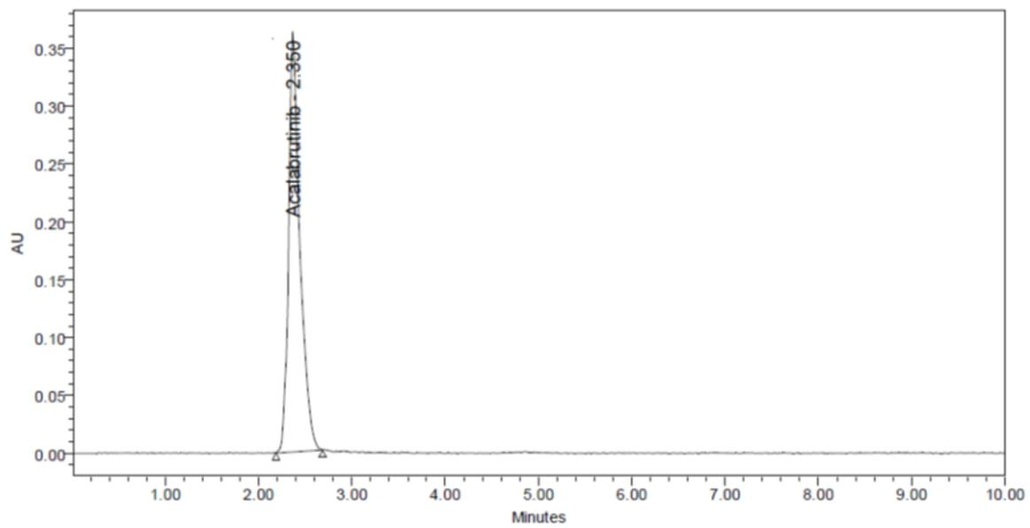
**Figure 12. Chromatogram of photo stability degradation of acalabrutinib**
