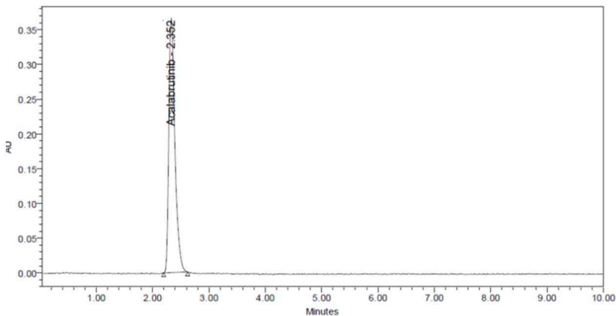
**Figure 8. Chromatogram of acidic degradation of acalabrutinib**
