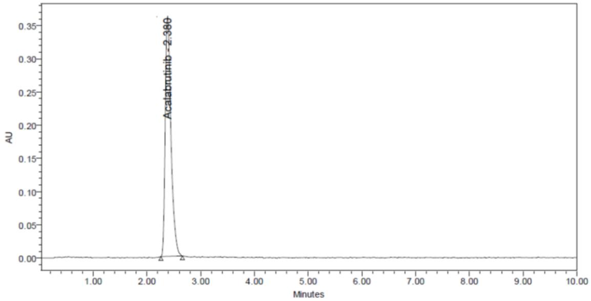
**Figure 11. Chromatogram of thermal degradation of acalabrutinib**
