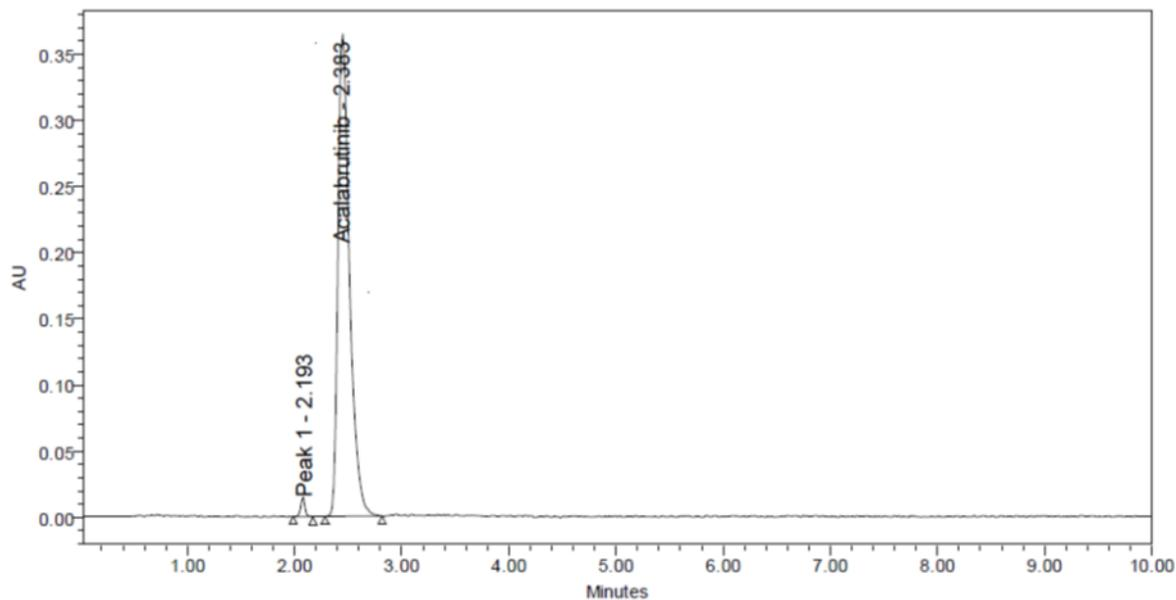
**Figure 9. Chromatogram of basic degradation of acalabrutinib**
