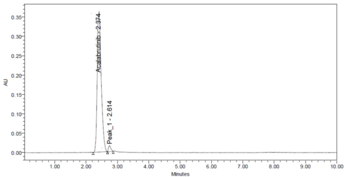
**Figure 10. Chromatogram of oxidative degradation of acalabrutinib**
