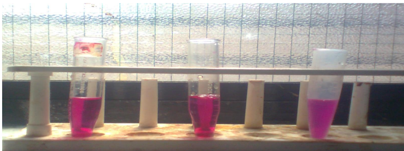
Figure No.8 : Estimation of undissolved \text{CaPO}_4 by titration method.
