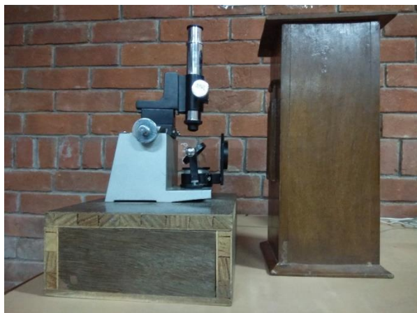
Fig. 1: Newton’s rings set up.
