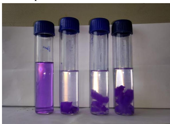
Figure 6: Adsorption of crystal violet dye on Poly (NTB-co-AM/MA) OMMT
