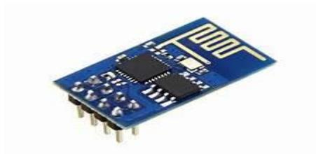
**Wi-Fi module-** Generally contains two main parts: a wi-fi chip and an application host processor.
