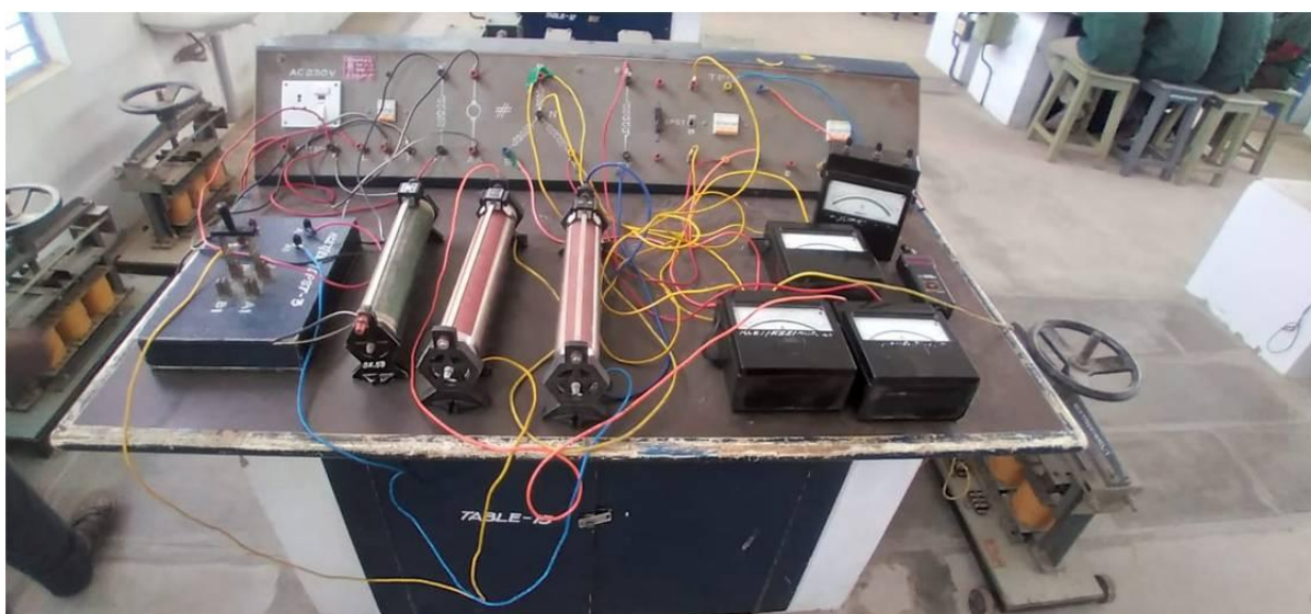
Fig: 3Hardware Connection of Alternator with inductive load
