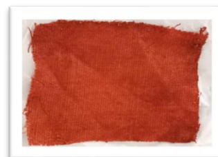
Plate- 5(b): Showing the colour of dye from Bixa orellana L. seeds when applying on cotton cloth
