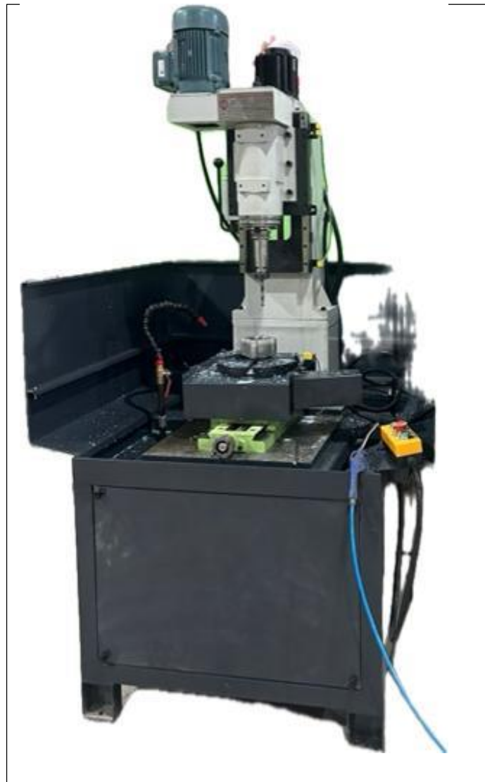
Fig 1. Automatic Peck Drilling Machine
