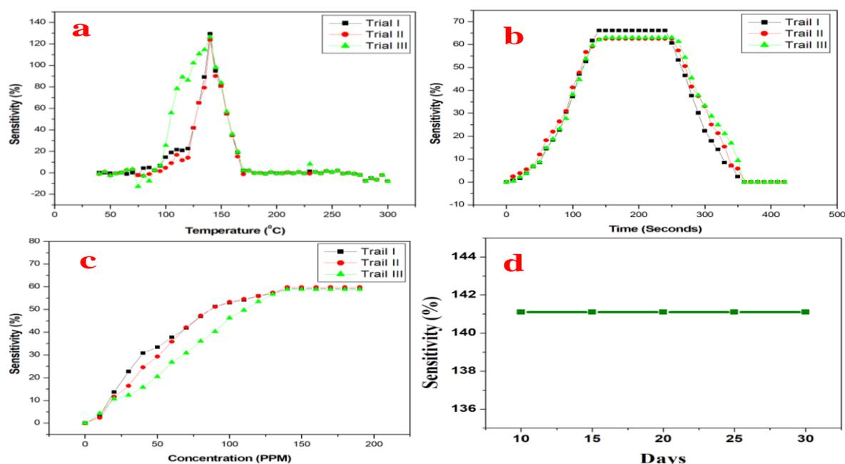
**Fig.2.** Sensing characteristics as (a) Operating Temperature (b) Response and Recovery time (c) Gas uptake capacity and (d) Stability of SnO<sub>2</sub> thick films
