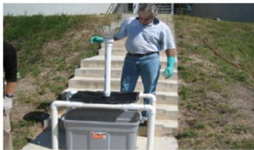
c) Geotextile dewatering test set up (GDT)
