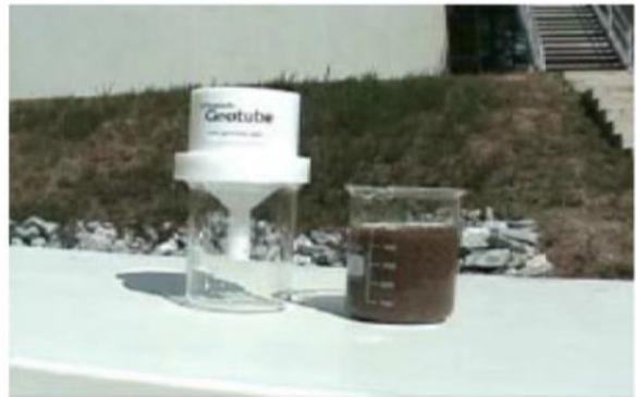
b) Rapid Dewatering test set up(RDT)
