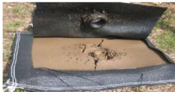
c) Geotextile dewatering test set up (GDT)
