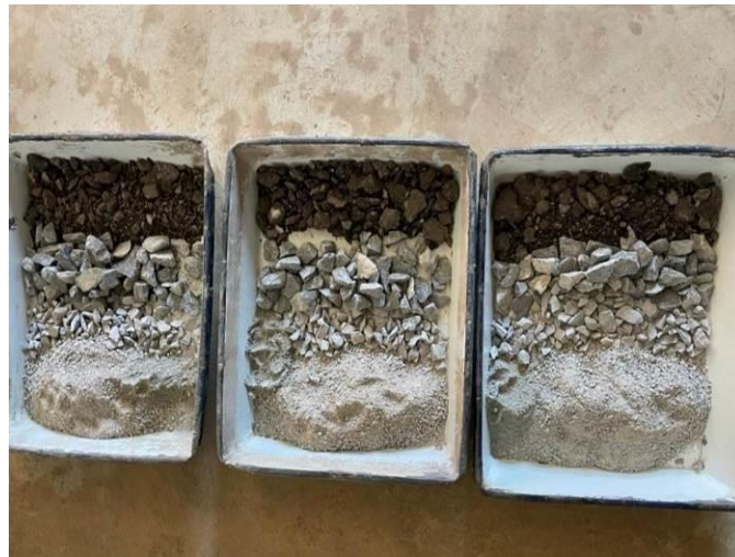
Figure.2.6 : Blending of aggregate with RAP
