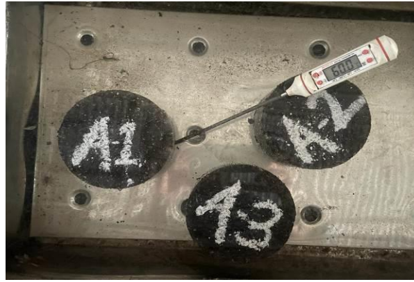
Figure 2.9 Arrangement of Water Bath at 60°C
