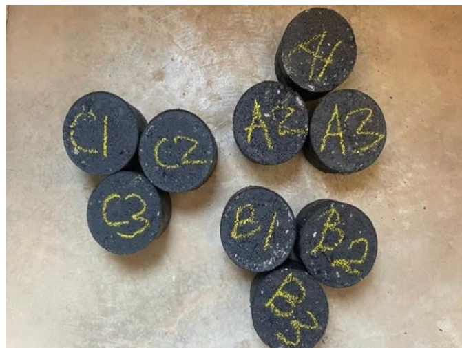
Figure 2.7: Samples for Marshal stability and Flow test.
