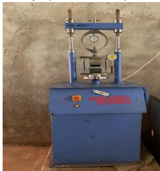
Figure 2.8 Marshall I Equipment
