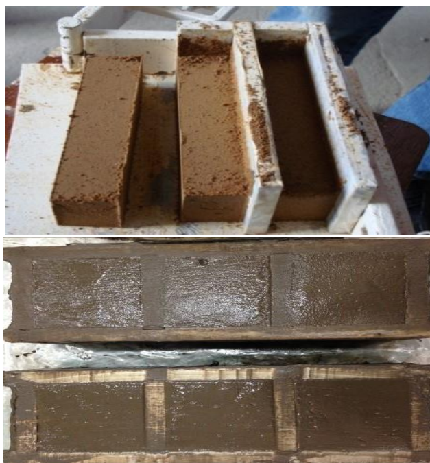
Fig.1.Geo-polymer specimens mold in preferred sizes
