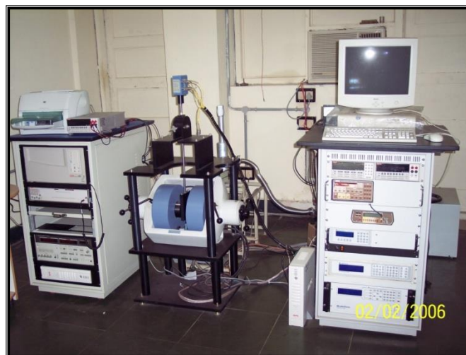
Figure 3 Lakeshore-7504 complete Hall effect measurement system.
