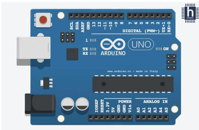
Fig. 6. Arduino Uno microcontroller
