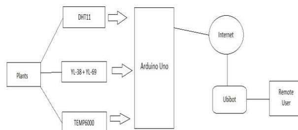
Fig. 2. Block diagram of the proposed architecture
