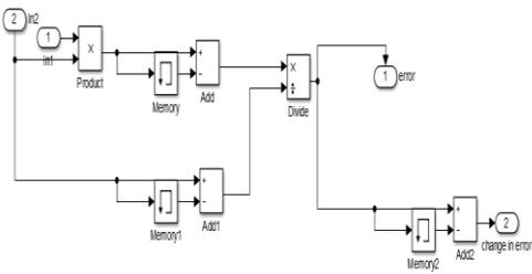
Figure 4: Subsystem for Power Error and Change in Error
