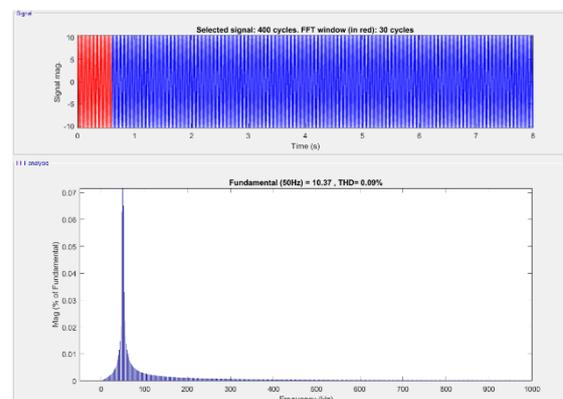
**Figure 10: THD output for Voltage**
