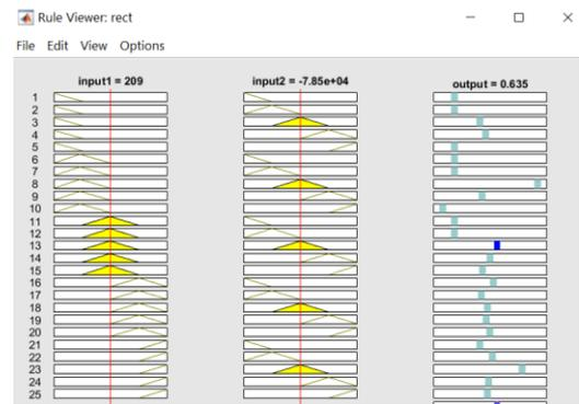
Figure 5: ANFIS Toolbox and rule view for Power Error and Change in Error and Output
