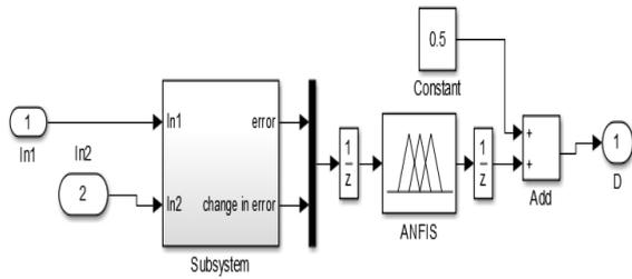
Figure 2: ANFIS Controller for Two PV inverters
