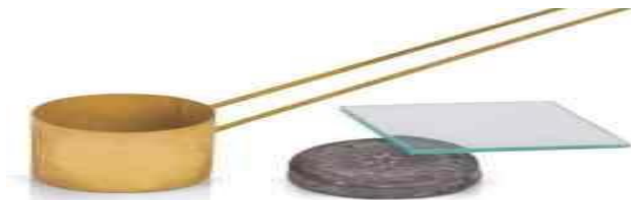
Fig3: Soundness of cement le chatlier's Test Apparatus
