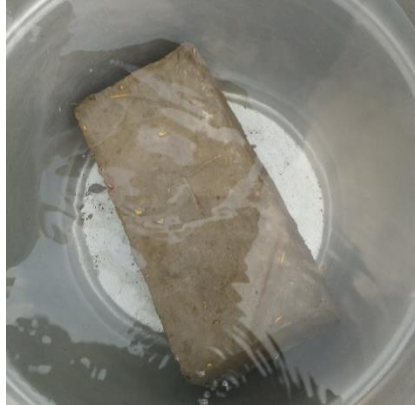
Fig 6: water absorption test
