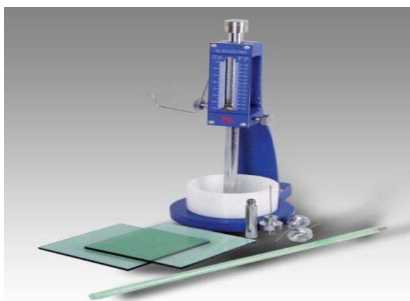
Fig 2: Vicat's Apparatus used for determination of setting time of cement
